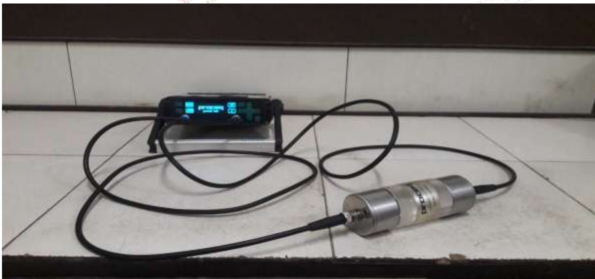
Fig. UPV Tester used in the Project
