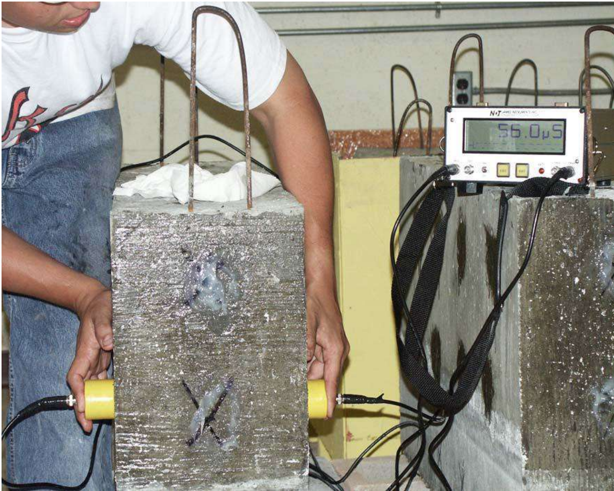
Fig. Testing of a beam by UPV Tester
