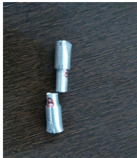
Fig. 3 Tensile test specimen after the test.
