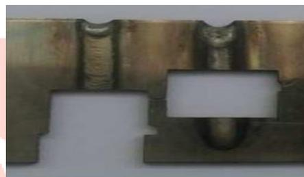
*Fig1 (b) specimen welded with Argon-hydrogen*
