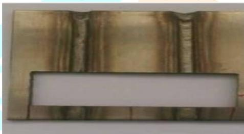
*Fig1(a) specimen welded with Argon*
