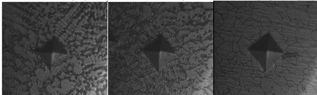
**Fig 5: (a)Indentation by vicker’s hardness tester on Ar welded samples.**
