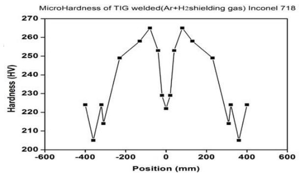
**Fig.4(b) Micro Hardness using Argon Gas-Hydrogen Gas**
