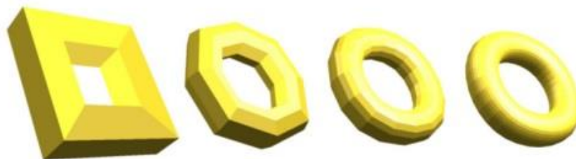
Fig 1: Subdivision recursively defines a smooth surface as the end of a succession of meshes.
