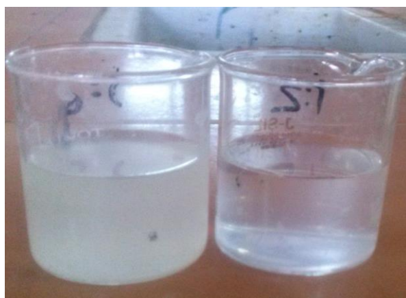
Figure 3: Wastewater sample (OPWW-sample-1) before and after algal treatment
