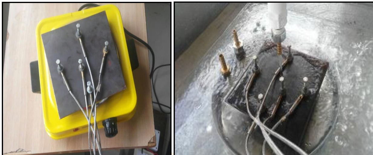
Figure 3. Heated copper Square Plate with arrangement of thermocouple
