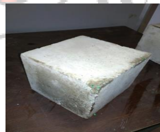
Fig. 2: Casted Concrete Block of Size 15cm 3 Using HDPE Granules
