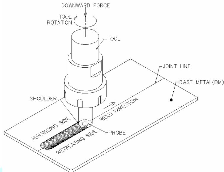
**Fig.1** The working principle of FSW
