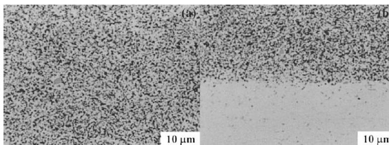
**Fig.5** Optical Micrographs showing (a) distribution of SiC particles ( 27 vol.%) in the aluminum alloy matrix, and (b) bonding of the surface composite and aluminum alloy substrate. (Misra et al., 2003)
