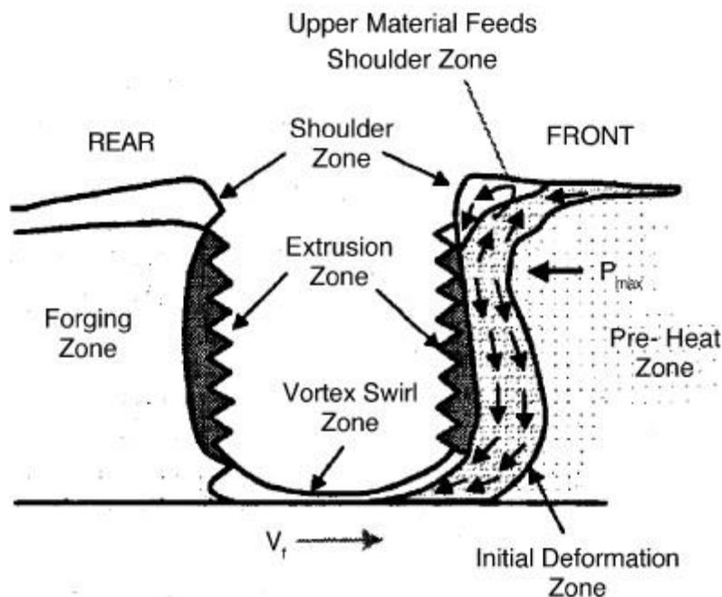
**Fig. 2** Material flow diagram in FSW
