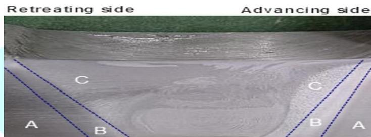
**Fig.3** Micro structural zone classification
