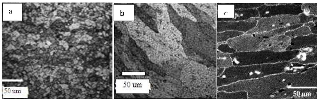
**Fig.4** Microstructure (a) SZ (b) TMAZ (c) HAZ.
