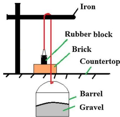
Fig. 3. Self-made adhesive strength test device
