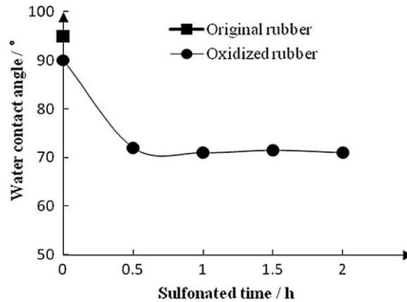
Fig. 5. Effect of sulphonated reaction on the contact angle of rubber surface with water
