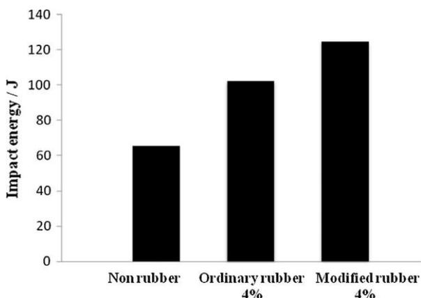
Fig. 9. The impact strength of different concretes.
