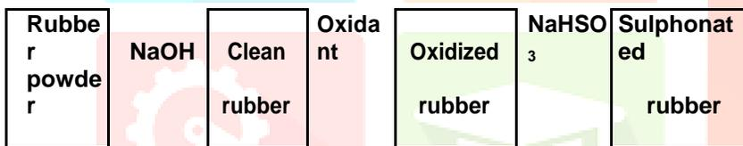
Fig. 1. Flowchart of the rubber modification process.
