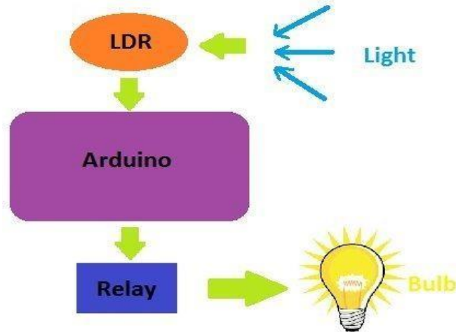
Figure: 6 LDR Sensor Mechanism
