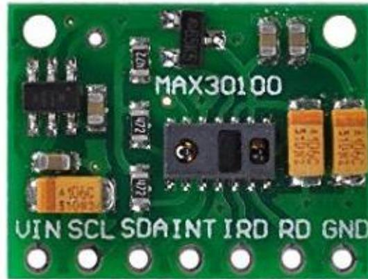
The sensor is integrated **pulse oximetry** and **heart-rate monitor** sensor solution. It combines two **LED's**, a **photodetector**, **optimized optics**, and low-noise analog signal processing to detect pulse and heart-rate signals. It operates from **1.8V** and **3.3V** power supplies and can be powered down through software with negligible standby current, permitting the power supply to remain connected at all times.
