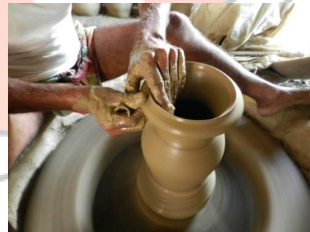
Fig. 5 Making the rim and collar
