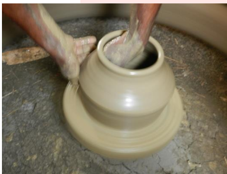
Fig. 4 Throwing (Thinning the wall)
