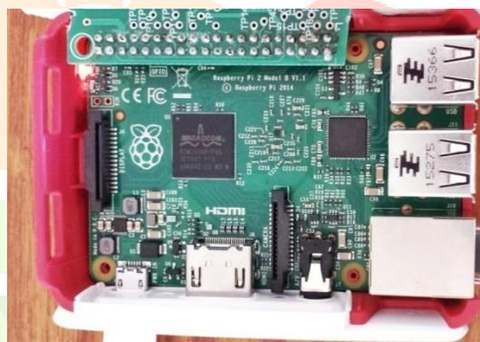
Fig 4: The Raspberry Pi board connected to a power supply and mounted GPIO ports
