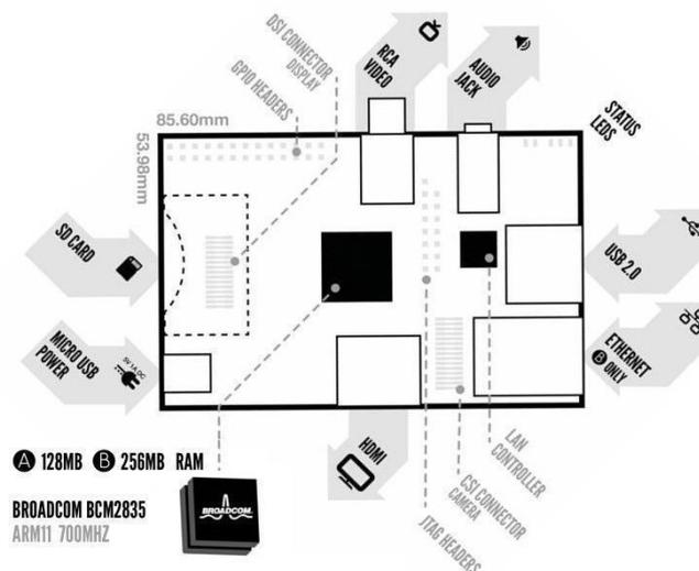
Fig 2: Raspberry Pi 2 setup
