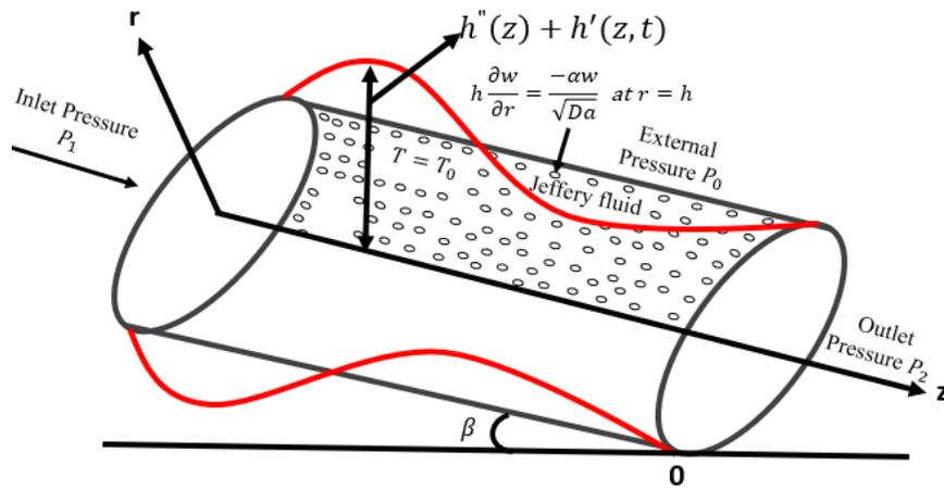
**Fig. 1. Geometrical representation of Peristaltic waves in an elastic tube.**
