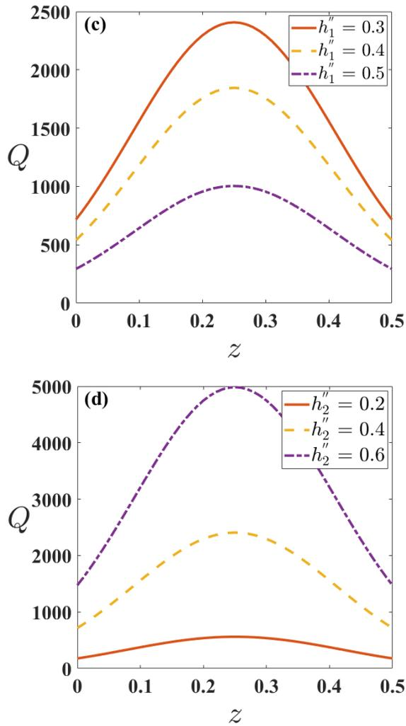
**Figure 3.**  $Q$  versus  $z$  for varying (a) elastic parameter ( $t_1$ ), (b) elastic parameter ( $t_2$ ), (c) inlet elastic radius ( $h_1''$ ) and (d) outlet elastic radius ( $h_2''$ )
