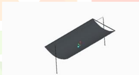
Fig:2 3D model of parabolic trough Diameter of parabolic trough-225mm Length -1115mm Stand height- 400 mm
