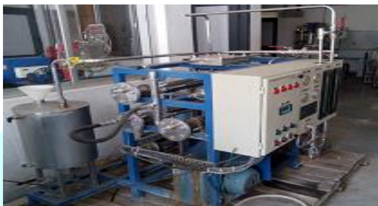
Figure 1. Reverse Osmosis Unit
