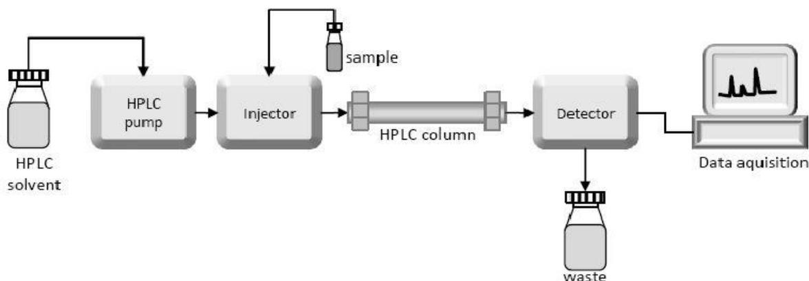
**a. Solvent Reservoir :** Mobile stage substance are contained in a glass reservoir. The versatile stage, or dissolvable, in HPLC is typically a blend of polar and non-polar liquid segments whose particular fixations are changed relying upon the arrangement of the specimen.
