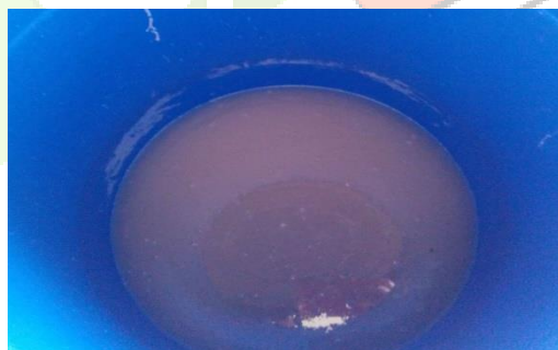
Solution of NaOH and Sodium Silicate
