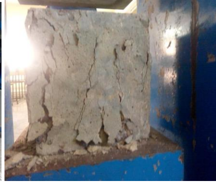
failure of cube
