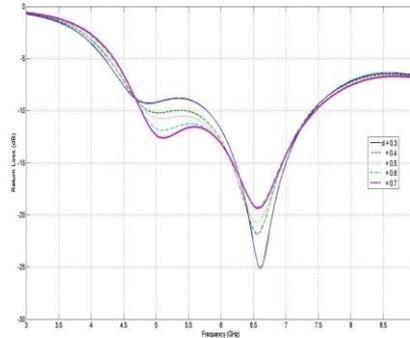
Fig.2. Return loss for variation of  $d$  (separation of feed strip from patch)
