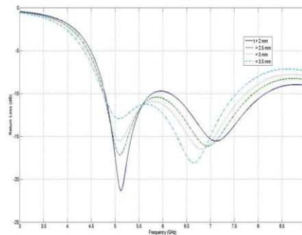
Fig.3. Return loss for variation of  $t$  (Width of feed strip)
