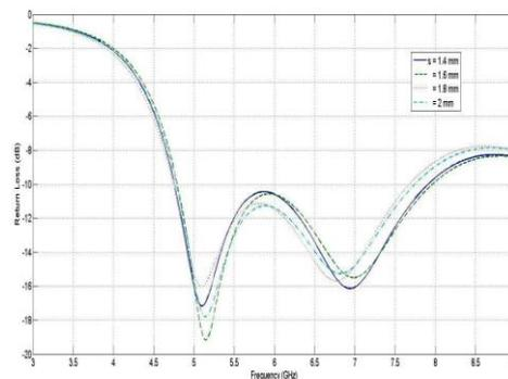
Fig.4. Return loss for variation of  $s$  (Length of feed strip)
