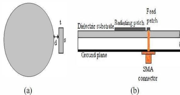
Fig.1. Feed Structure (a) top view (b) side view
