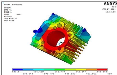
Fig.21. Temperature Distribution through curved fin 3mm
