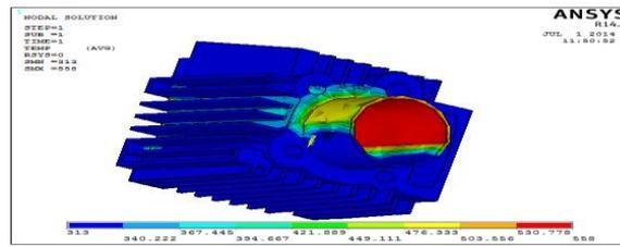
Fig.12. Temperature Distribution through Rectangular fin2.5mm thickness)
