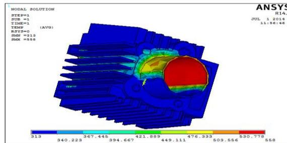
Fig.14. Temperature Distribution through Rectangular fin2.5mm thickness)
