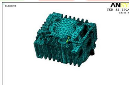
Fig.4. Mesh model of rectangular fin(2.5mm thickness)
