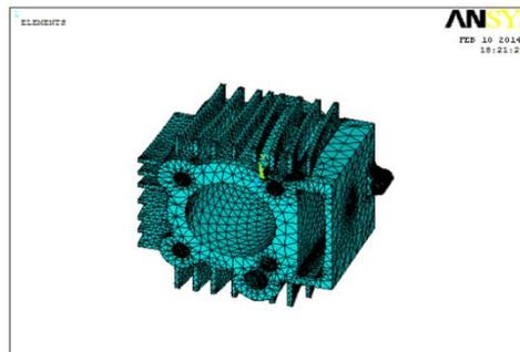
Fig.6. Mesh model of circular fin(3mm thickness)
