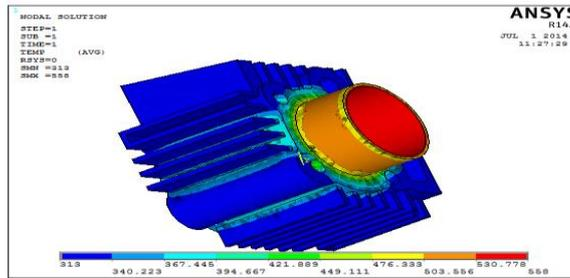
Fig.13. Temperature Distribution through Rectangular fin3mm thickness)
