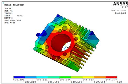
Fig.19. Temperature Distribution through curved fin 3mm
