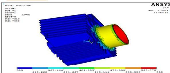
Fig.9. Temperature Distribution through Rectangular fin 3mm thickness)
