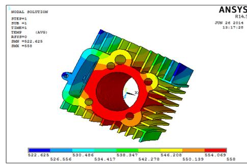
Fig.20. Temperature Distribution through curved fin 2.5mm
