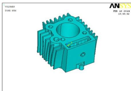
Fig.5. Pro/E model of curved fin (3mm thickness)
