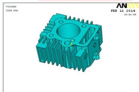
Fig.3. Pro/E model of rectangular fin (2.5mm thickness)
