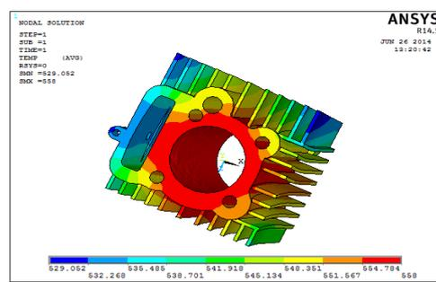
Fig.22. Temperature Distribution through curved fin 2.5mm
