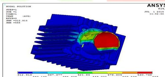
Fig.10. Temperature Distribution through Rectangular fin 2.5mm thickness)
