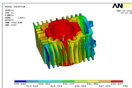
Fig.18. Temperature Distribution through curved fin2.5mm
