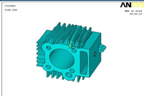
Fig.7. Pro/E model of curved fin (2.5mm thickness)
