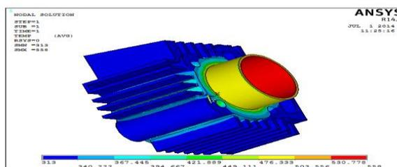
Fig.11. Temperature Distribution through Rectangular fin 3mm thickness)
