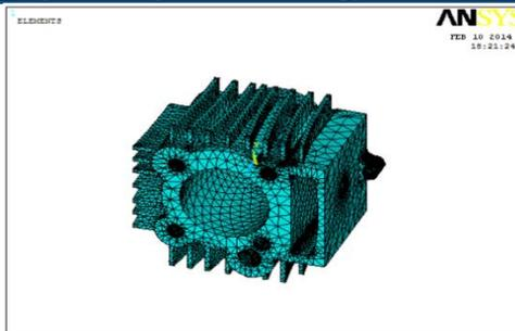
Fig.8.Mesh model of curved fin(2.5mm thickness)
