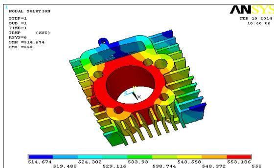
Fig.17. Temperature Distribution through curved fin3mm
