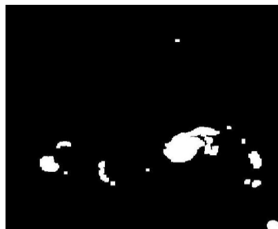
Fig 2.4 Binary image after the morphological opening operation
