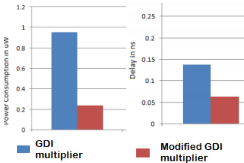
Fig 8: Power and delay comparison of modified GDI multiplier with conventional GDI multiplier
