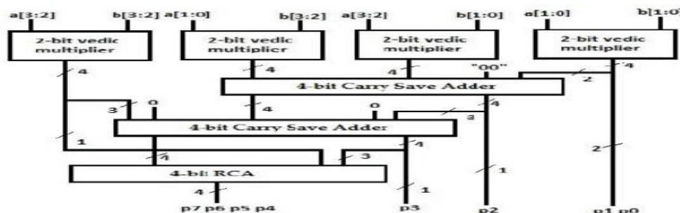
Fig 5: Block diagram of 4x4 vedic multiplier
