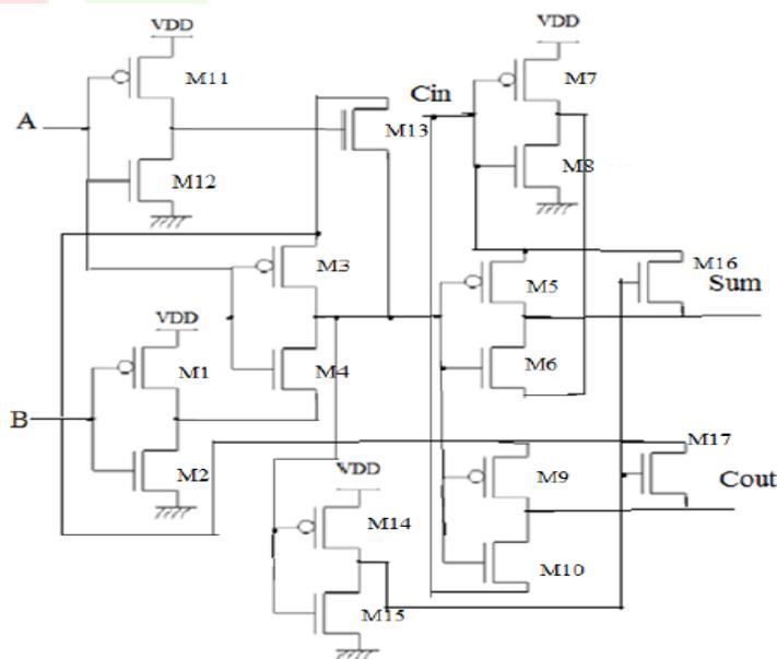
Fig 3: 1-bit Full adder using full swing modified GDI technique
