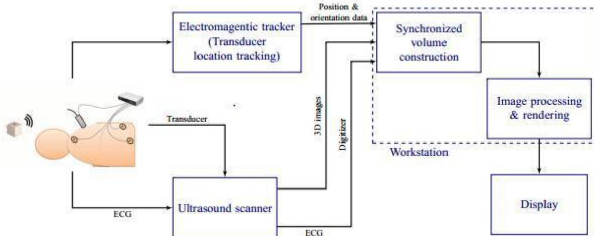
Fig 1. The proposed system show the tracking system for multi-view echocardiography
