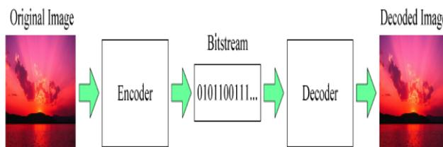
**Fig 1.Basic flow of image compression coding.**
