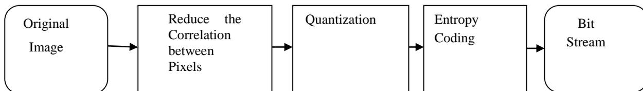
**Fig. 2. General encoding flow of Image compression**
