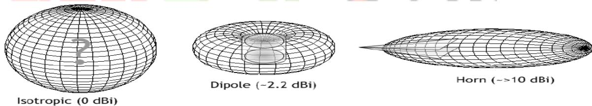
Fig 1.1: An isotropic antenna has a gain of 0 dBi by definition. A small dipole antenna typically has a gain of about 2.2 dBi, and a horn antenna may have a gain of 10 dBi or more.
