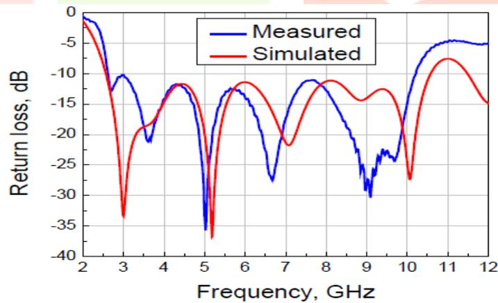
Fig 4.7: Measured and simulated return loss curves of microstrip line fed elliptical slot antenna
