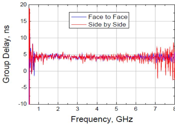
Fig 4.6: Group delay of measured transfer function of vertical disc monopole pair
