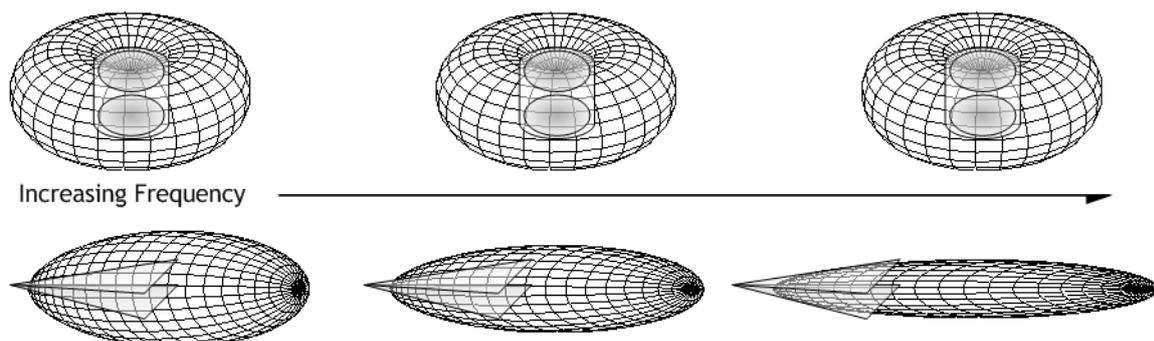
Fig 1.2: The pattern of a constant gain antenna remains fixed with increasing frequency (top), while the pattern of a constant aperture antenna narrows and gain increases with increasing frequency.
