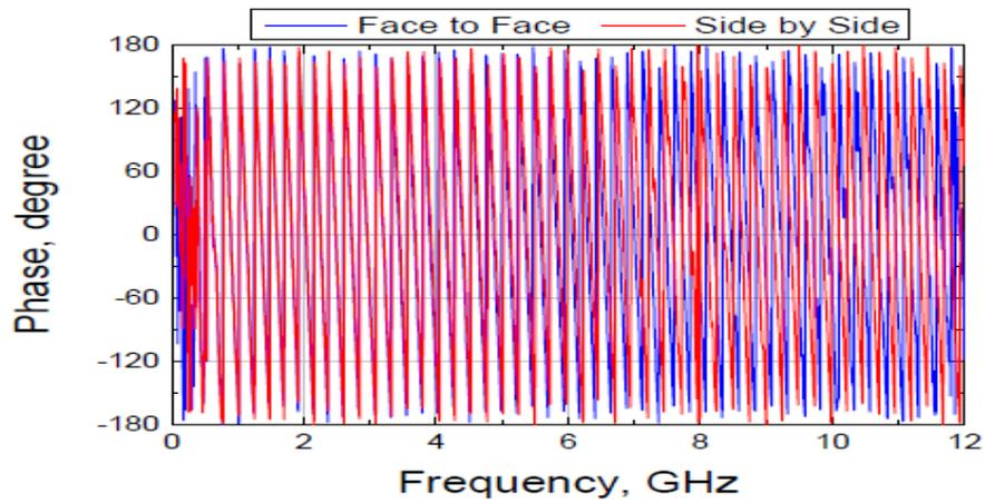
Fig 4.5: Phase of measured transfer function of vertical disc monopole pair
