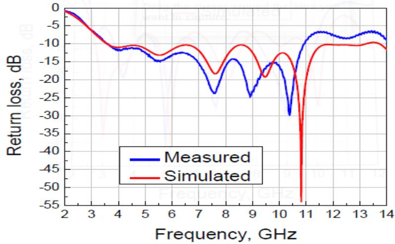
Fig 4.8: Measured and simulated return loss curves of microstrip line fed circular slot antenna
