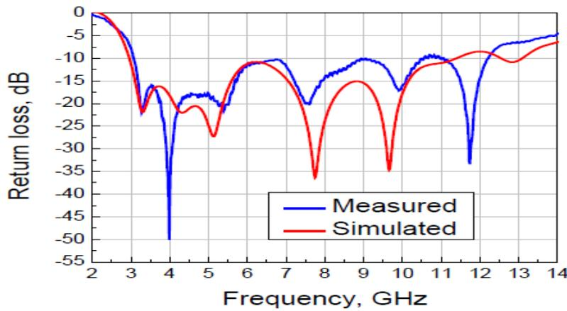
Fig 4.9: Measured and simulated return loss curves of CPW fed elliptical slot antenna
