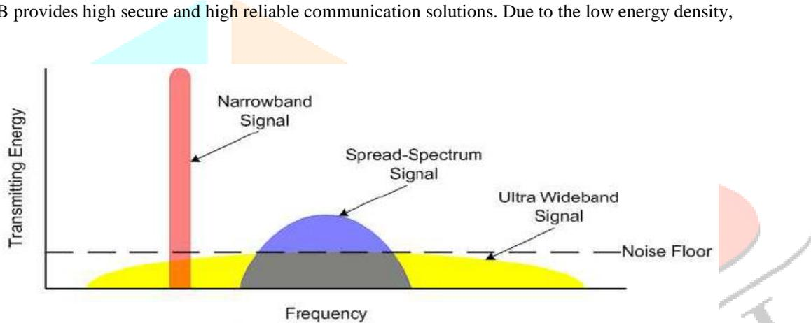
Fig 5.1: Ultra wideband communications spread transmitting energy across a wide spectrum of frequency
