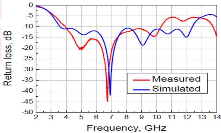
Fig4.10: Measured and simulated return loss curves of CPW fed circular slot antenna
