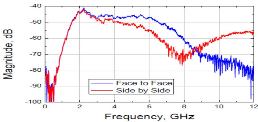
Fig 4.3: Magnitude of measured transfer function of vertical disc monopole pair
