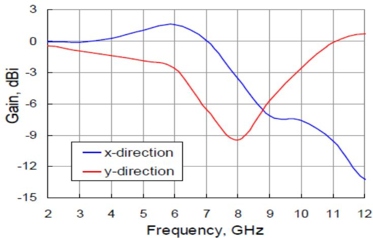
Fig 4.4: Simulated gain of vertical disc monopole in the x -direction and the y-direction
