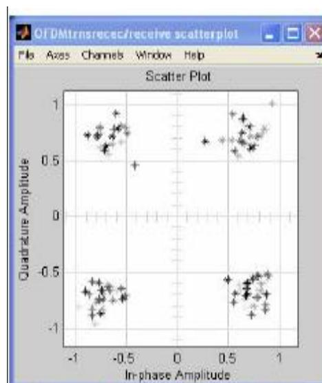
(b) Received signal with phase distortions
