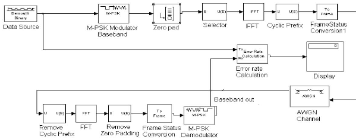
Figure 1. Block diagram of OFDM transceiver
