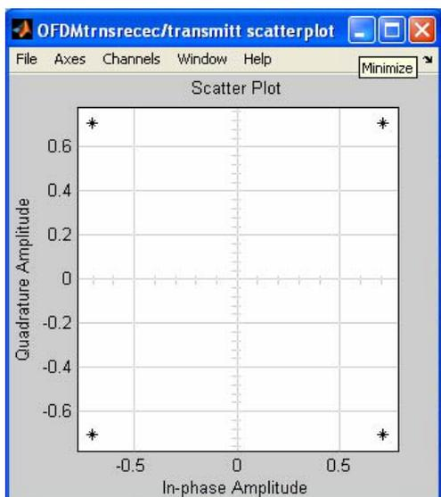
(a) Transmitted signal with 4 phases
