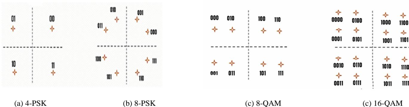
Figure 2. Constellation diagrams 4/8-PSK and 8/16-QAM
