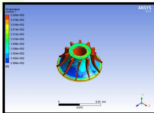
Figure 8.2.3 Results of Temperature flow inside the turbine
