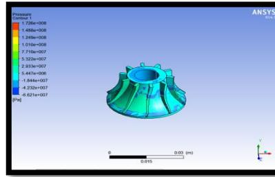
Figure 8.1.1 Result of pressure flow inside the turbine
