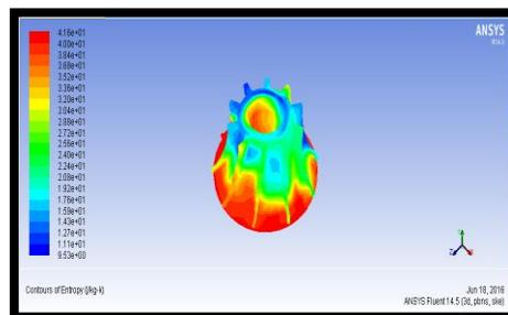
Figure 8.1.4 Results of Entropy flow inside the turbine
