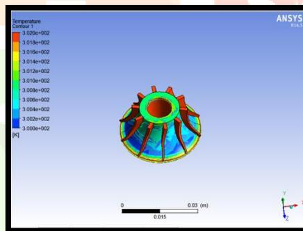
Figure 8.13 Results of Temperature flow inside the turbine
