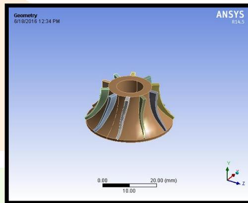
Figure4.1 Sample Model designed with using blade angle  $15^\circ$
