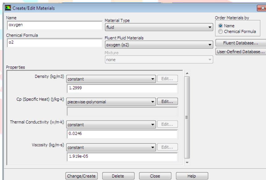
Figure 7.3 Fluid conditions for oxygen
