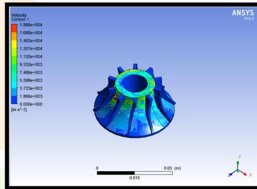
Figure 8.2.2 Results of velocity flow inside the turbine
