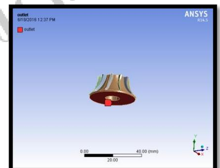
Figure4.3 Outlet fluid passage
