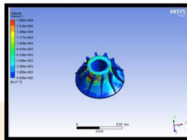
Figure 8.2.1 Results of velocity flow inside the turbine
