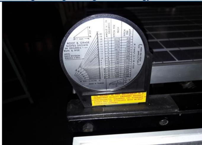
fig.9 Tilt angle indicator in solar PVTR system
