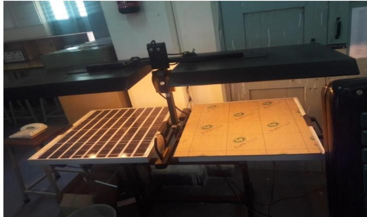
Fig.6 single panel completely shaded
