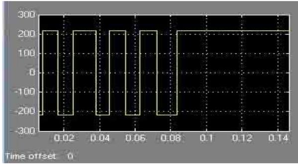
**Transformer Secondary Winding Voltage**
