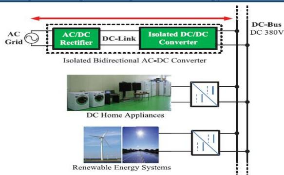
Fig.1.1 380-V Dc Distribution System With An Isolated Bidirectional AC–DC Converter
