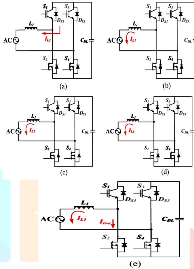
**Fig. 5. Operating modes in the rectifier's generation mode using the same switching pattern as the rectification mode: (a) Mode 1, (b) Mode 2, (c) Mode 3, (d) Mode 4, and (e) Mode 5.**
