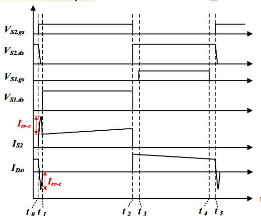
**Fig.3.2. Theoretical operating waveforms of the proposed bidirectional ac–dc rectifier in the rectification mode.**
