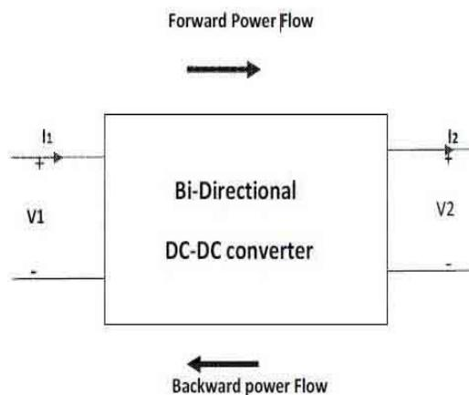
Fig.5- 1 Illustration of bidirectional power flow
