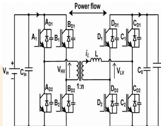
Fig 4.1 Schematic of the DAB DC-DC Converter
