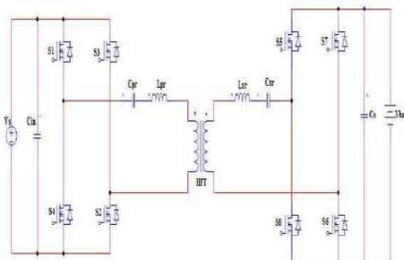
Fig 6.1 Full-bridge series resonant converter
