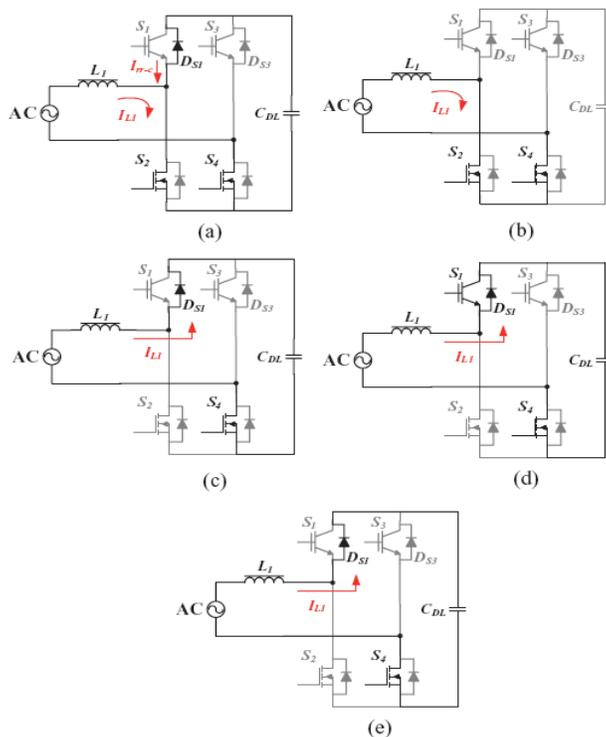
**Fig.3.1 Operating modes of the proposed bidirectional ac–dc rectifier in the rectification mode: (a) Mode 1, (b) Mode 2, (c) Mode 3, (d) Mode 4, and (e) Mode 5**
