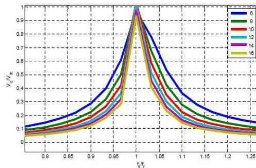
Fig. 6.2: Characteristics of SRC resonant converter
