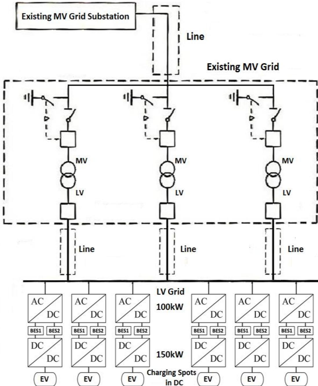
Figure 4.2:DC fast charging station in mode 4 with BESs connected to LV
