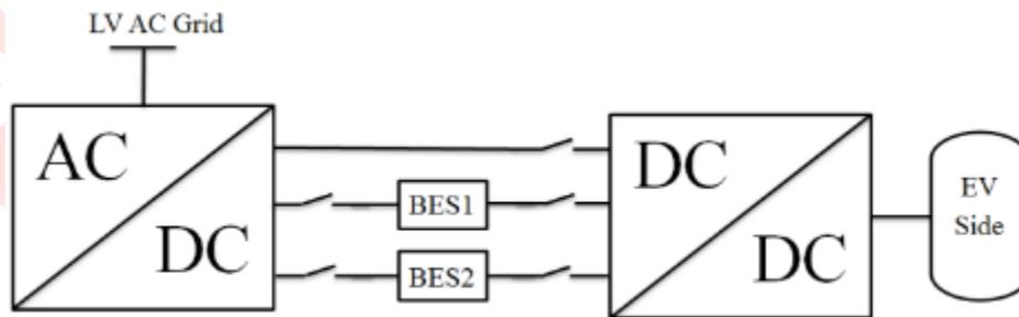
Figure 4.4:DCfast charging station in LV grids with BESs
