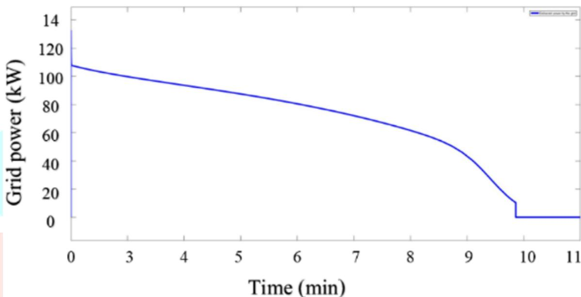
Figure 5.1:Active power delivered by the LV grid
