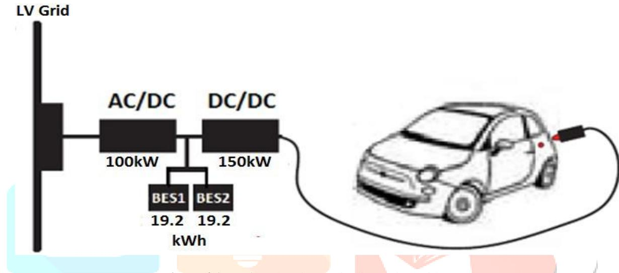
**Figure 4.1:**DC fast charging station in mode 4 with BESs
