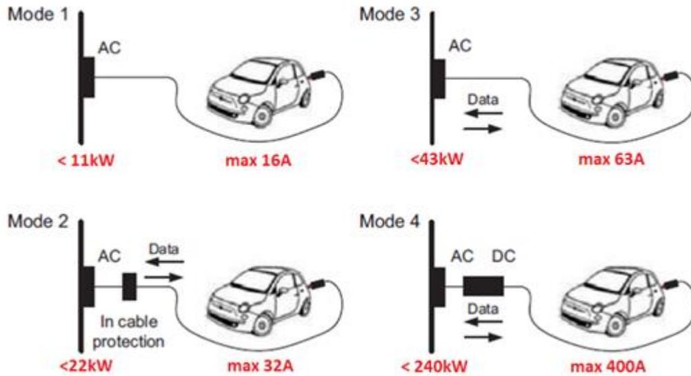
Figure 4.3:DC - Fast charging station in mode 1, 2, 3 and 4
