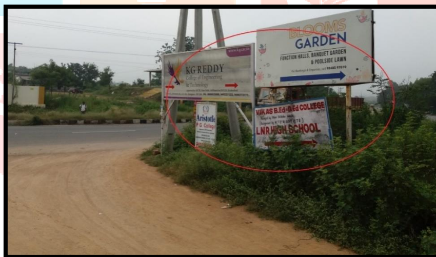
Fig 13 Route indicating boards causing blind spots.
