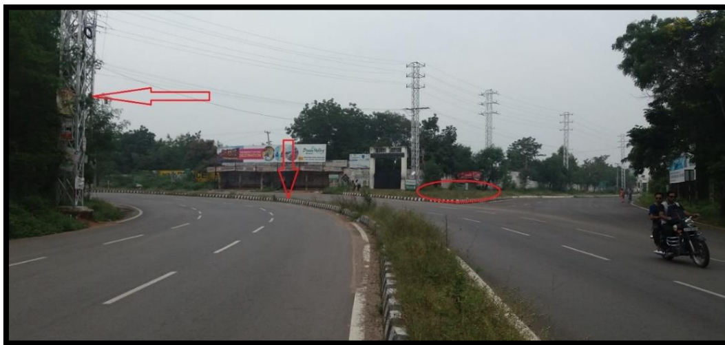
Fig 5 signing boards were not placed to guide the turning.
