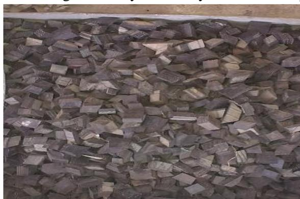
**Fig 1. Rubber Aggregates (20mm)**
