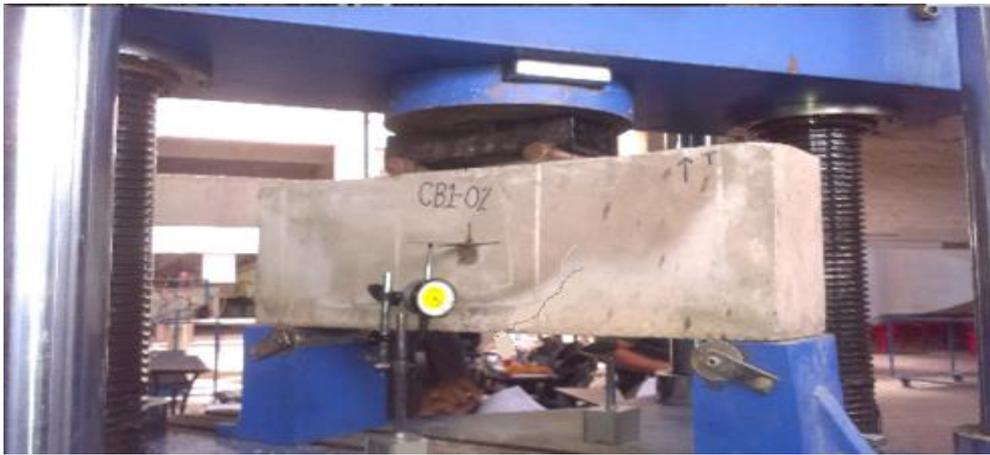
**Figure 5** Shows failure of beam with flexural crack at centre
