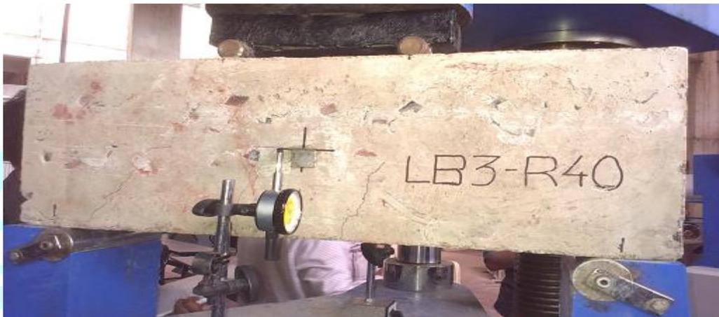
**Figure 6** Shows shear crack at supports and flexural cracks at center
