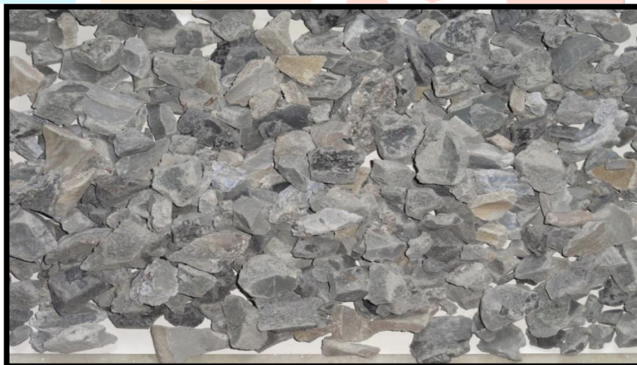
Fig. 2 Waste Polymer Aggregates (WPA) derived from Jali Gola .
