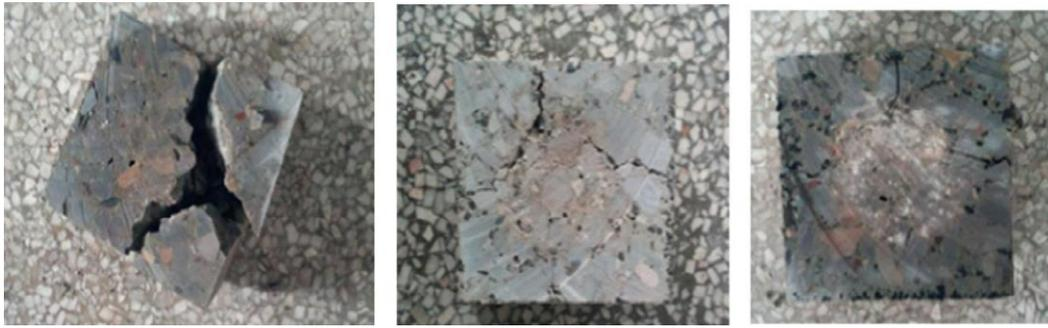
Fig. 10. Failure modes of concrete specimen subjected to ultimate impact.
