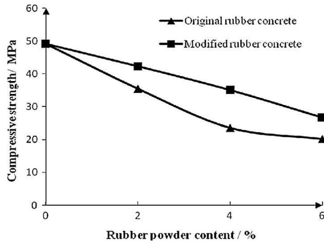
Fig. 8. Relation between rubber content and compressive strength.
