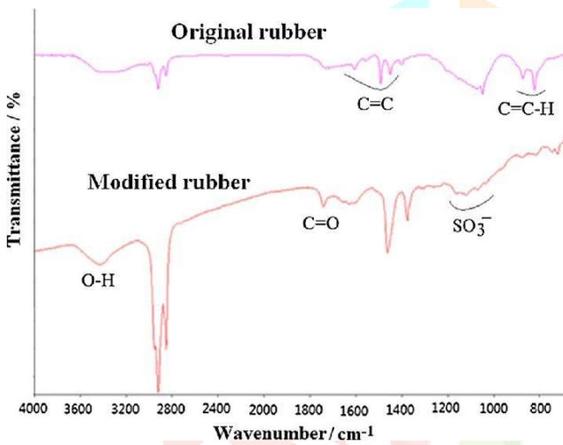
Fig. 6. FT-IR spectra of crumb rubber before and after modification.
