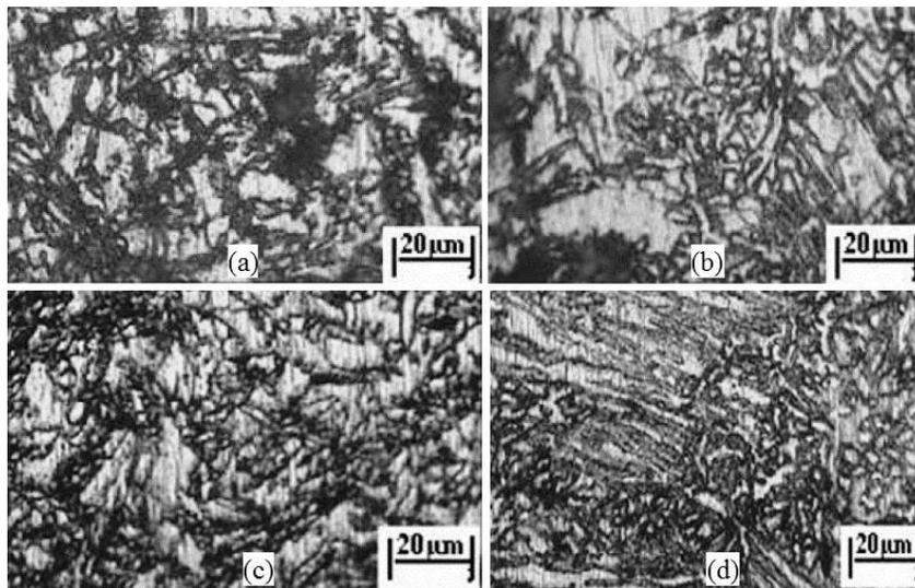
Fig. 4 (a) Ar-shield weld metal, (b) Ar-shield heat affected zone, (c) He-shield weld metal (d) He-shield heat affected zone
