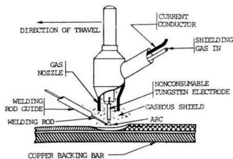
Fig. 1. TIG Welding mechanism
