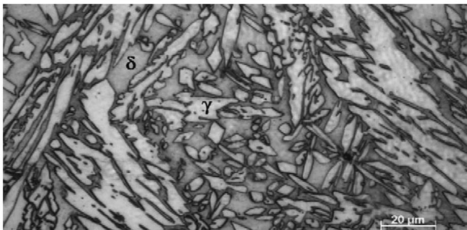
Fig. 2 Fusion area in LAM steel
