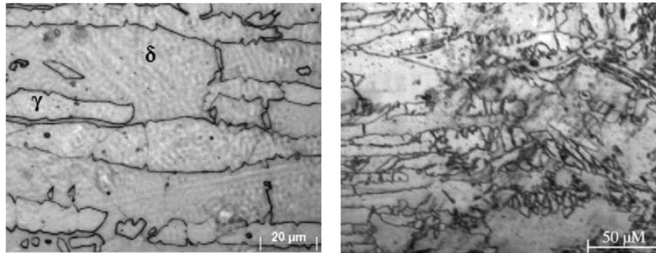
Fig. 3 Structures of (a) partially annealed and (b) overheated part of the HAZ
