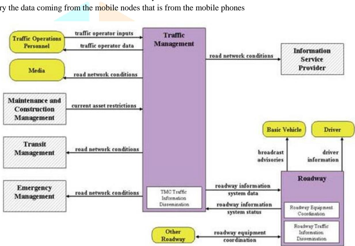
Figure 9: Schematic of the workings of a TMC [6]
