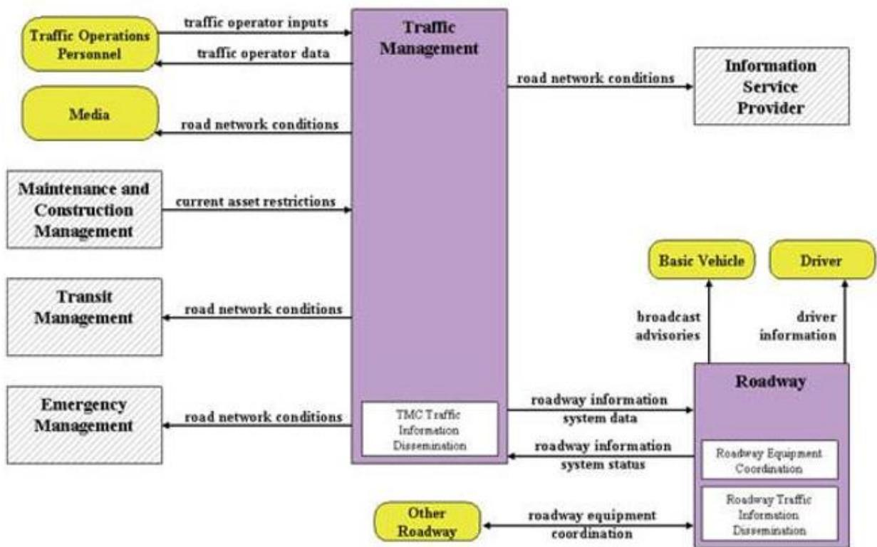
Figure 9: Schematic of the workings of a TMC [6]
