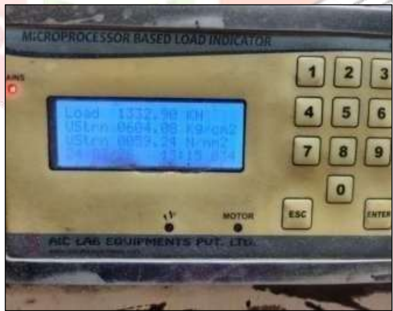
Fig.09. Cube Testing at Knack Laboratory at Vadala
