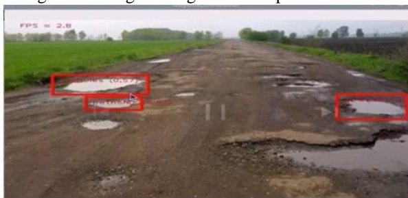
Fig. Processing of image to detect potholes
