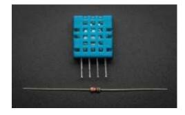
The DHT11 is a basic, ultra low-cost digital temperature and humidity sensor. It uses a capacitive humidity sensor and a thermistor to measure the surrounding air, and spits out a digital signal on the data pin (no analog input pins needed). Its fairly simple to use, but requires careful timing to grab data. The
