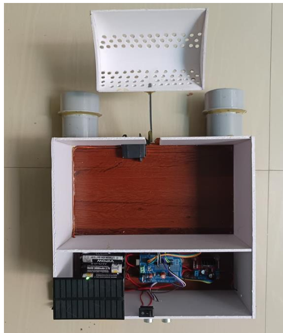
Fig. 2: Prototype Implementation of the Solar-Powered Automated Electronic Waste Sorting System
