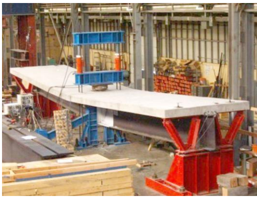
a) beam tests
