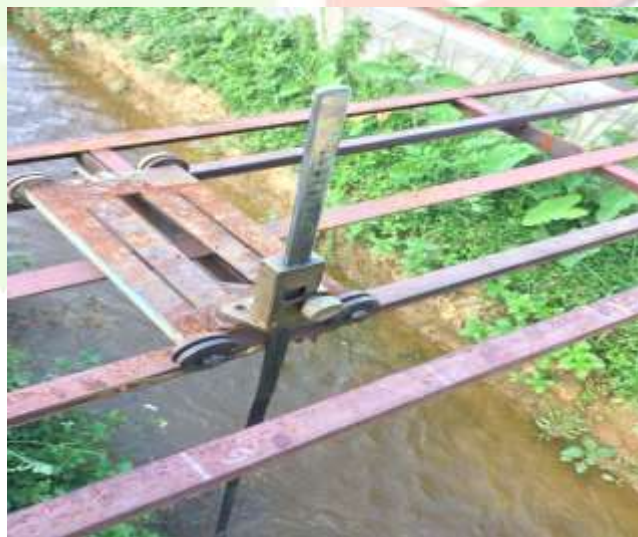
Fig 8: Installed point gauge with steel trolley
