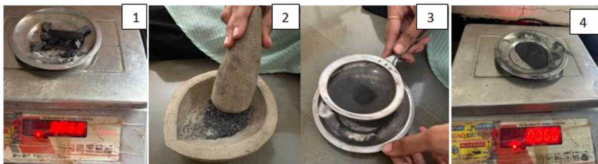
Figure number. 1: Weighing of Shuddaloha, 2: Trituration of ShuddaLoha, 3: Sieving of Triturated Shudda Loha Churna, 4: Weighing of obtained Shudda Loha SukshmaChurna.
