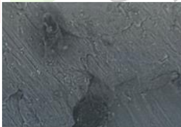
Fig. 6.5d: At 5% SiC, SiC particles were uniformly embedded with minimal defects, affirming effective reinforcement-matrix bonding.
