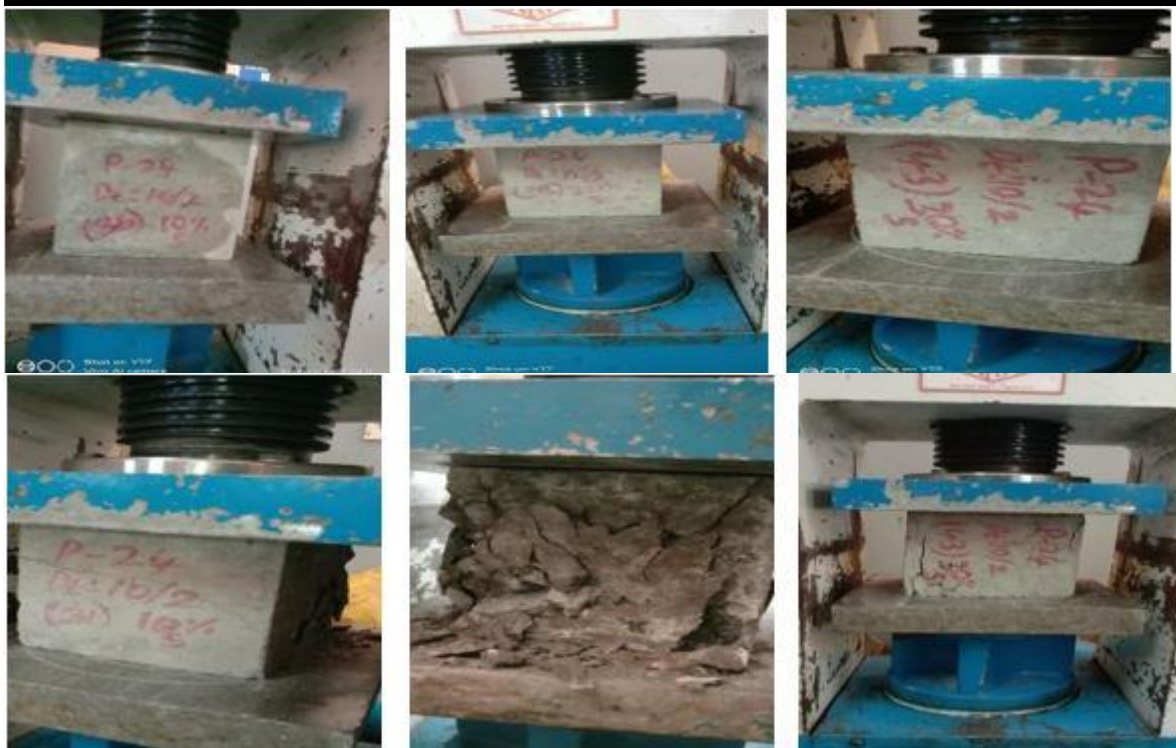
FIG NO: 3.6 BEFORE & AFTER CRACK FOR REPLACEMENT OF F.A. BY STEEL SLAG
