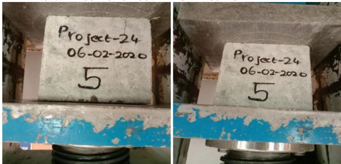
FIG NO: 3.2 BEFORE & AFTER CRACK OF CONVENTIONAL CUBES
