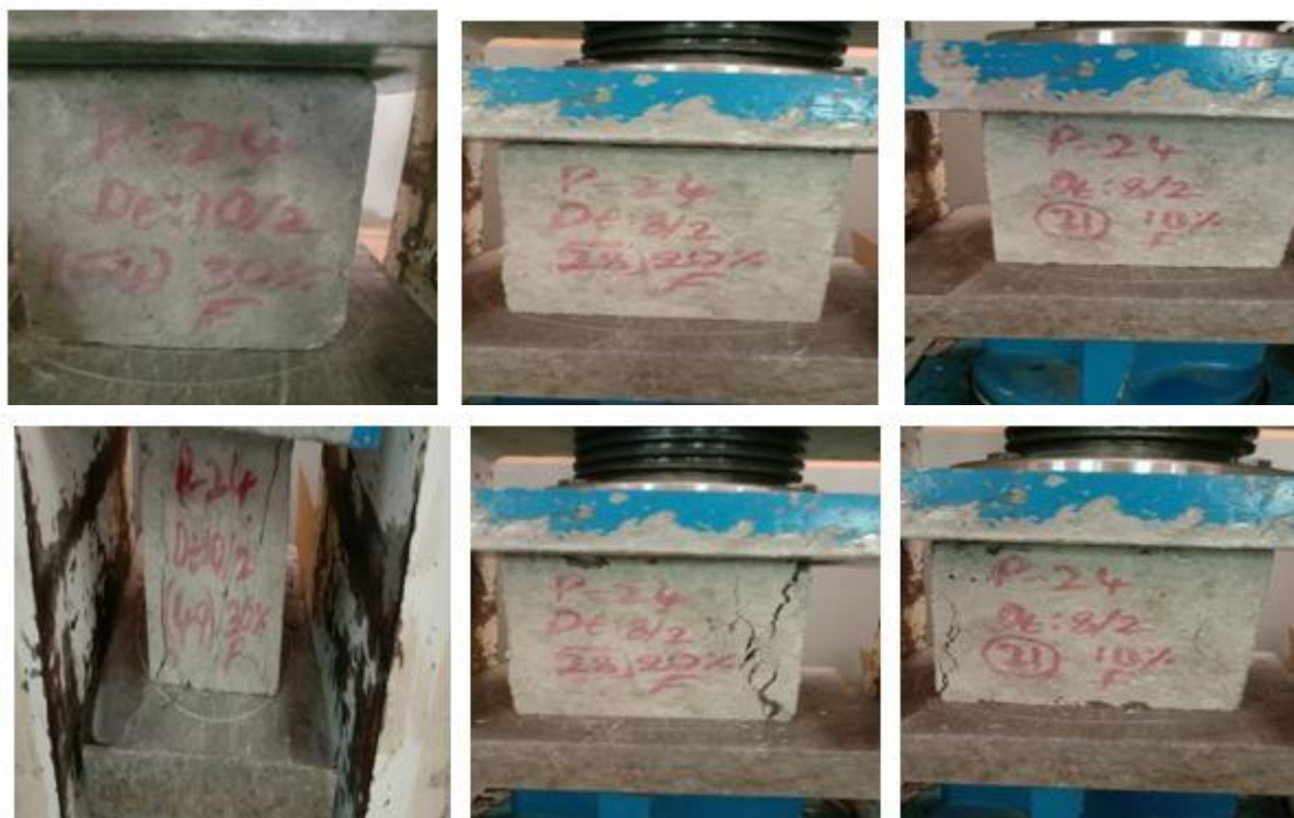
FIG NO: 3.4 BEFORE & AFTER CRACK FOR REPLACEMENT OF CEMENT BY FLY ASH
