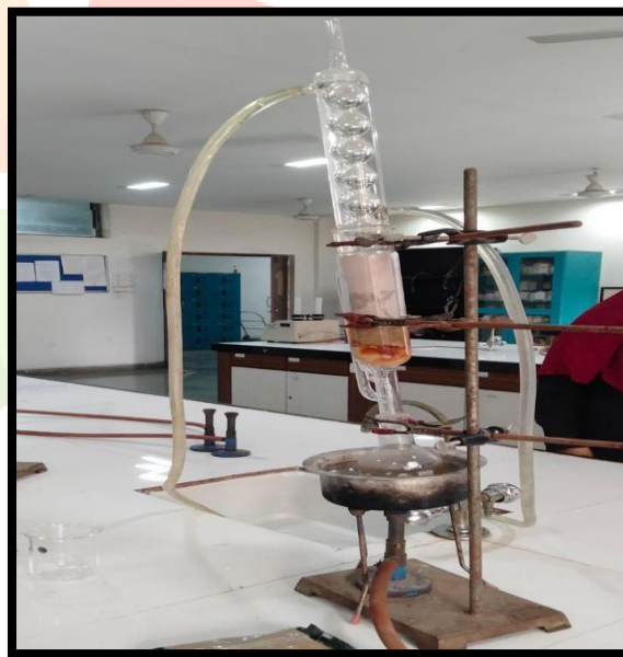
FIGURE 11 SOXHLET EXTRACTION PROCESS
