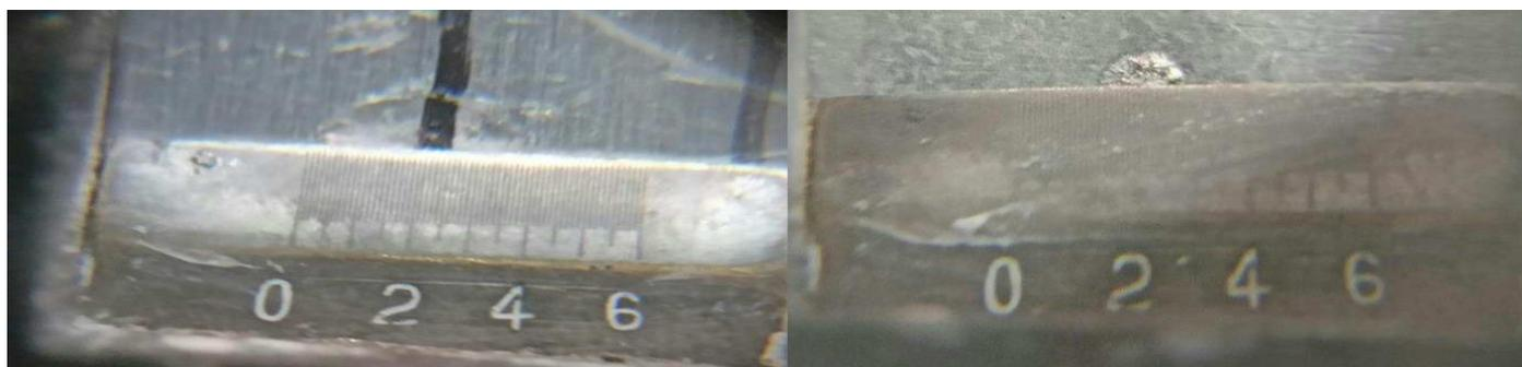
**Figure 5: nuggets diameter and spot formation of Sample – II**
