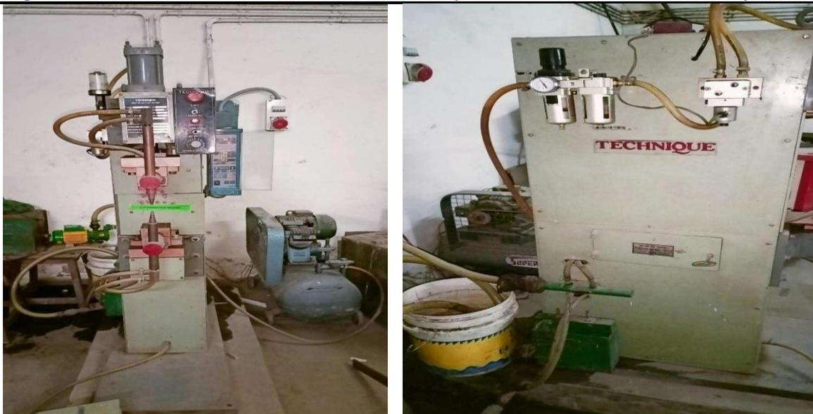
Figure 3: Spot welding machine
