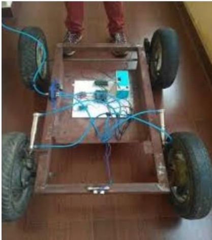
Fig. 1: Ultrasonic sensor and MC Unit mounted on motorcar
