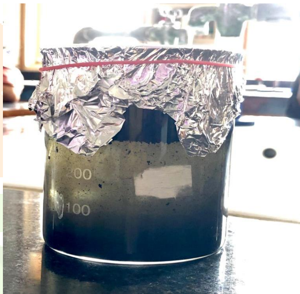
fig.3.8: Impurities and charcoal separation
