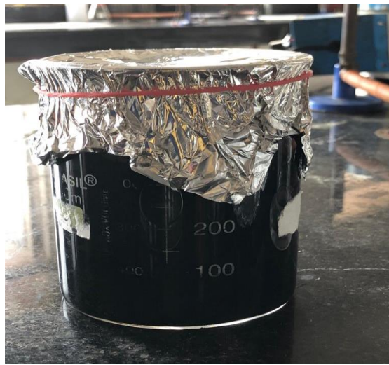
fig.3.7: Charcoal in \text{CaCl}_2 solution
