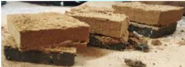
Fig 4.3 Sample III – Clay + Sawdust
